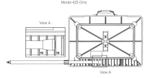
Adjust all 4 legs to desired length before assembling to the table.
